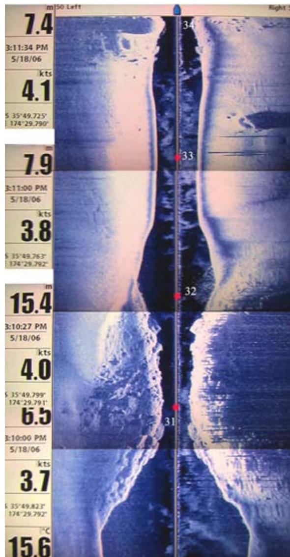
**Figure 7.** Representative sonar images. This image is a composite of a series of screen shots on a survey line from sonar points 31-34 (refer Map Section Map 1). This track runs from south to north just past the west end of Motukaroro Island. The distance from data point 31 to point 34 is 181 m.
