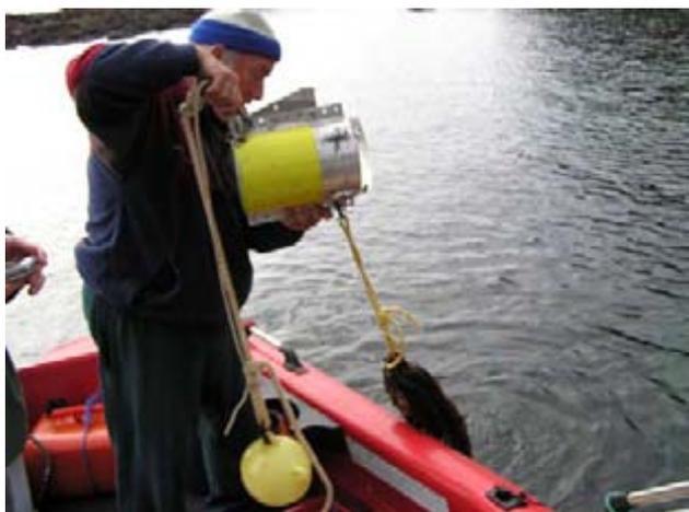
**Figure 4.** Drop video apparatus
