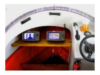
Figure 5. Sonar equipment and research boat
