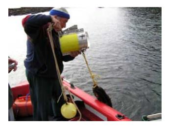
Figure 4. Drop video apparatus
