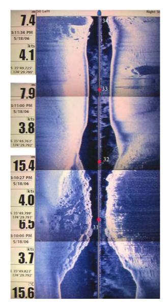
**Figure 7.** Representative sonar images. This image is a composite of a series of screen shots on a survey line from sonar points 31-34 (refer Map Section Map 1). This track runs from south to north just past the west end of Motukaroro Island. The distance from data point 31 to point 34 is 181 m.
