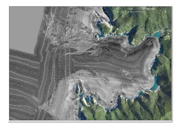
**Figure 4** OS 20/20 sonar multibeam backscatter layer displayed over a contour hillshade bathymetry layer. The grayscale in this imagery displays the hardness or softness of the sea bottom substrate. Dark areas are sandier and lighter areas are shell, gravel or reef.
