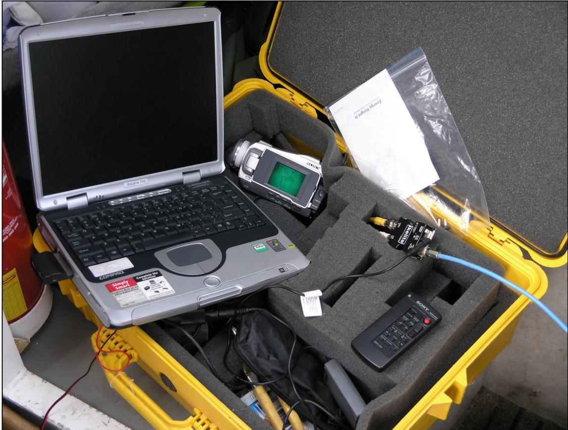
**Photo 23. Collection apparatus consisting of a line feed from the underwater camera (blue cable) feeding an Ikelite power and data manager, feeding a Sony video camera where still images are captured onto a memory stick. The video camera is connected to the laptop via a fire-wire cable allowing direct capture and immediate digitising of video footage.**
