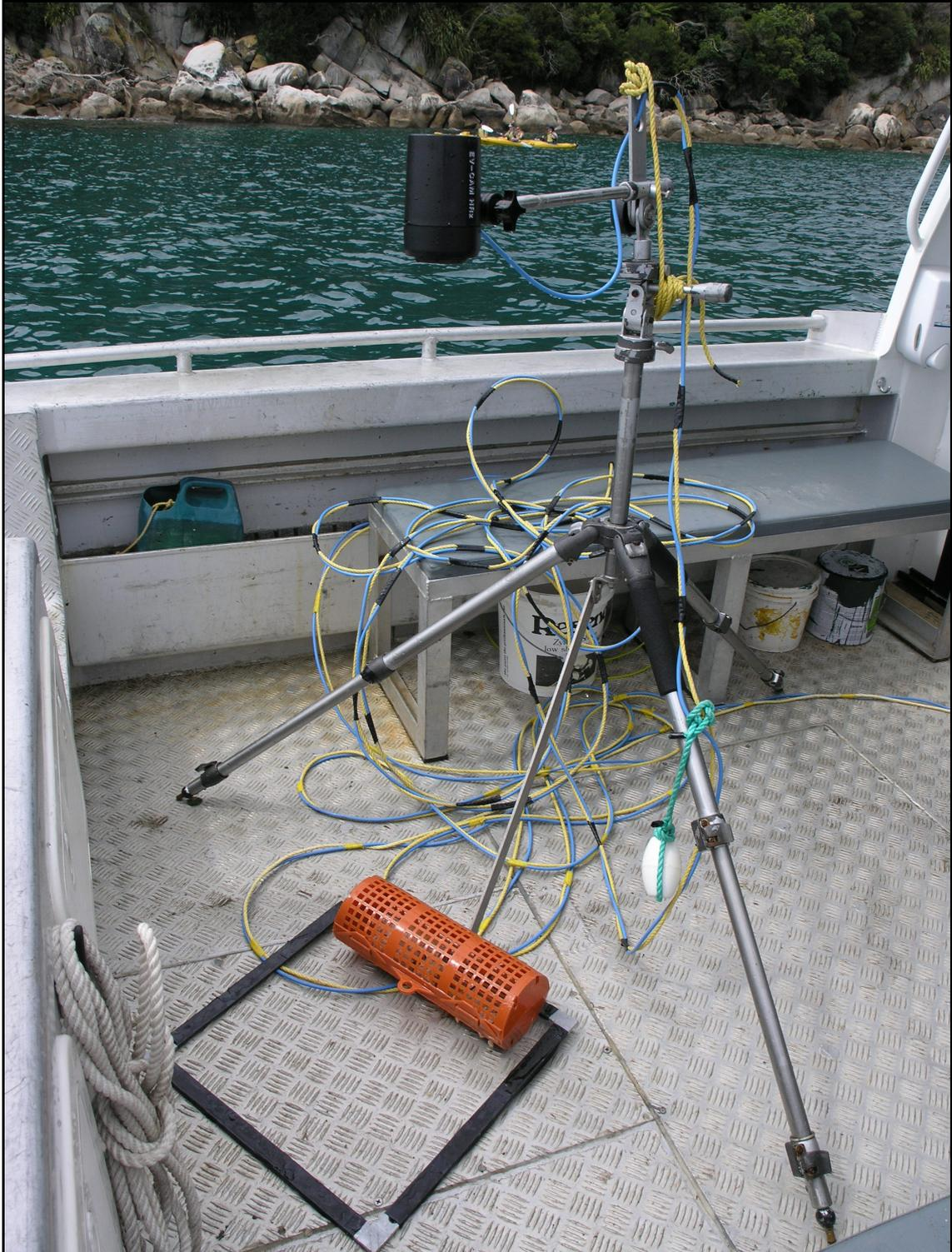
**Plate 1. BUV apparatus consisting of a modified tripod with attached reference square and commercial bait container.**
