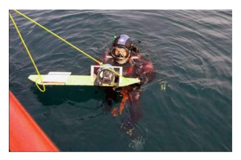
Figure 5 Manta board fitted with video camera
