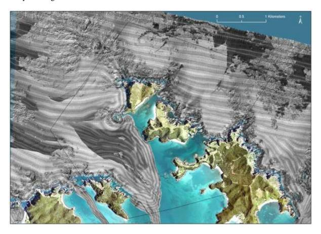
Figure 7 OS 20/20 multibeam backscatter layer displayed over a contour hillshade bathymetry layer. The thin black line depicts the mapping area.
