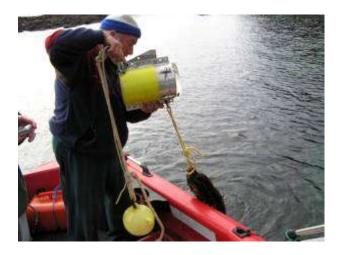
Figure 3 Drop video system, (second system).
