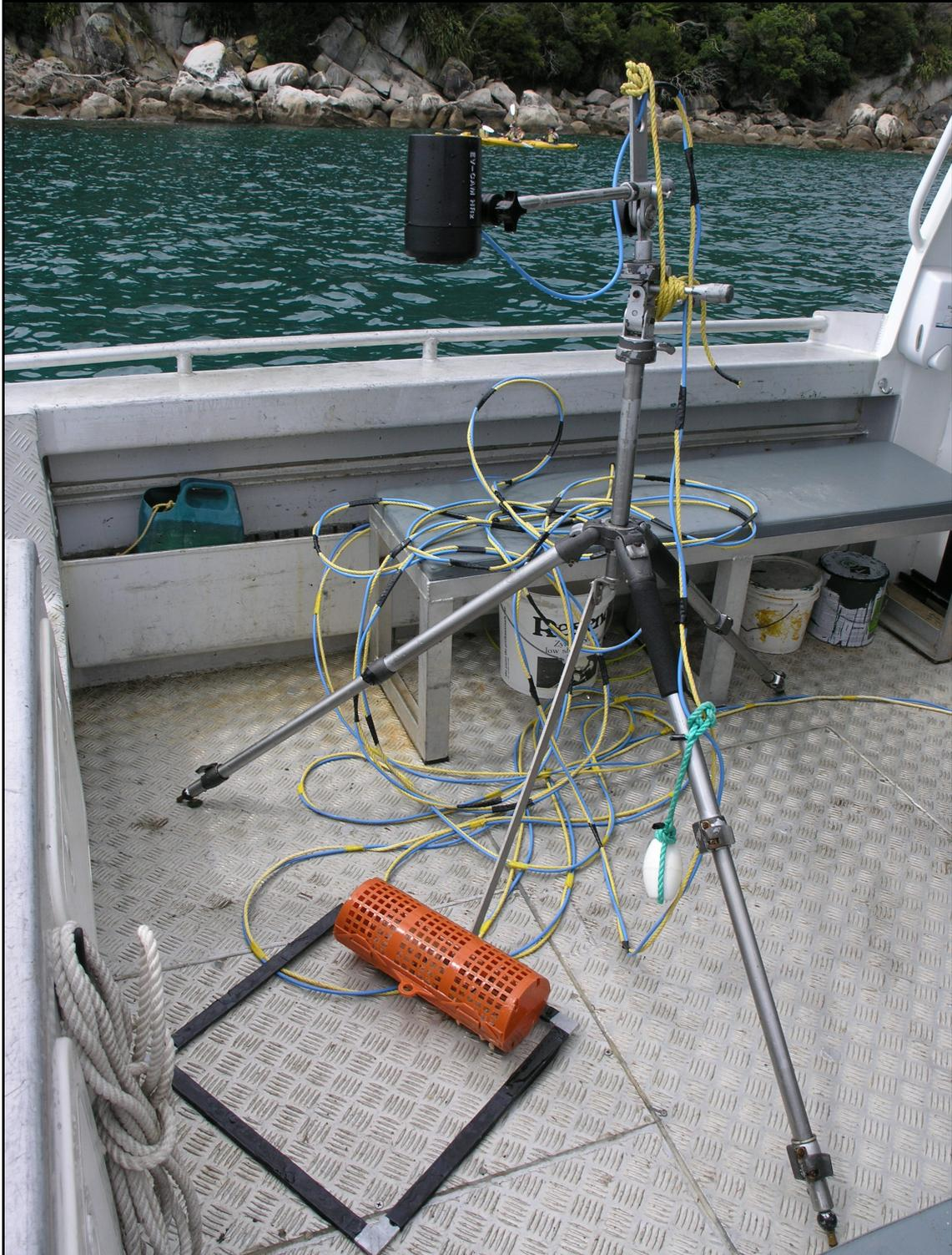
**Plate 1. BUV apparatus consisting of a modified tripod with attached reference square and commercial bait container.**
