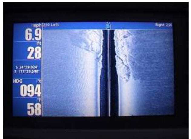
Fig. 8. Double-sided sidescan image running from sand at the bottom to low relief rock toward the top.
