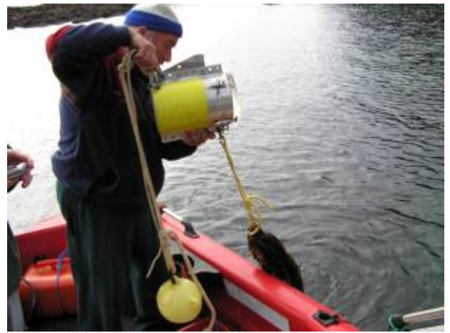
Fig. 6. The drop-video apparatus being lowered over the side of the 4.2m Mac boat.
